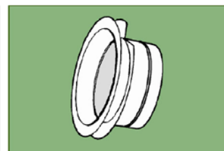
Figure 29 Ductboard Collar (Spin-In)
